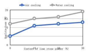
Fig. 5. The influence of chemical additive on the quality loss of foam concrete
