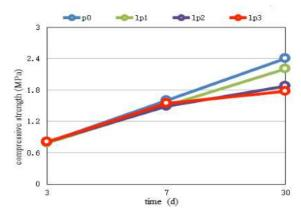
Fig. 3. The influence of chemical additive on the compressive strength of foam  $\operatorname{concrete}$
